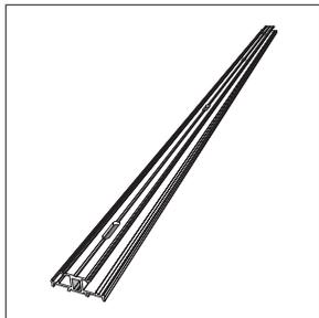
This coupling side guiding channel has pre-drilled slots (5 mm x 20 mm) at every 250 mm. Please maintain a maximum distance of 500 mm between two attachment points.
